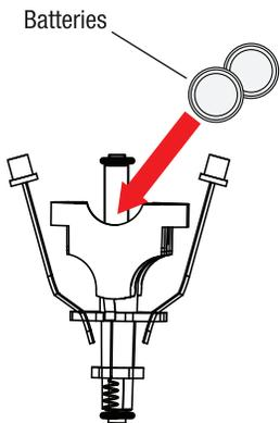
6. Replace with new batteries in the same +/- orientation as the old batteries.
