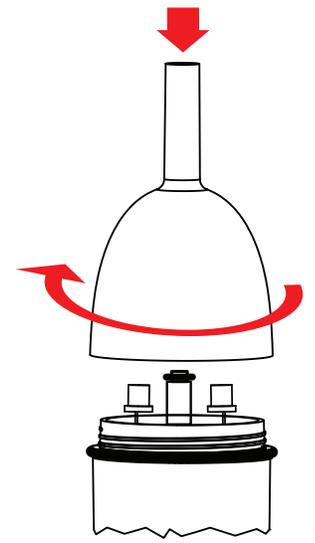
10. Screw on top of float snugly without over tightening.
