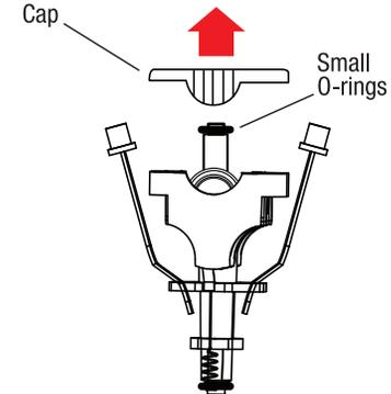
4. Gently pull cap off battery assembly by pulling straight up.
