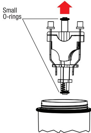
2. Carefully remove battery assembly, pulling straight up from bottom of float.
