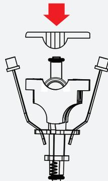
7. Replace cap onto battery assembly. Press firmly into place.
