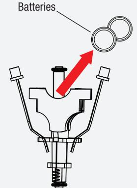
5. Remove old batteries from assembly noting +/- orientation.
