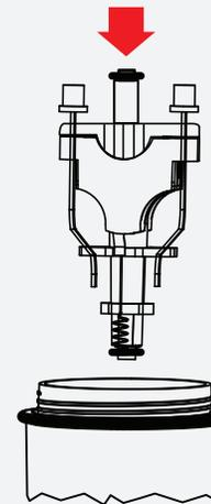
9. Reseat battery assembly into bottom of float aligning the assembly with the guides inside of float.
