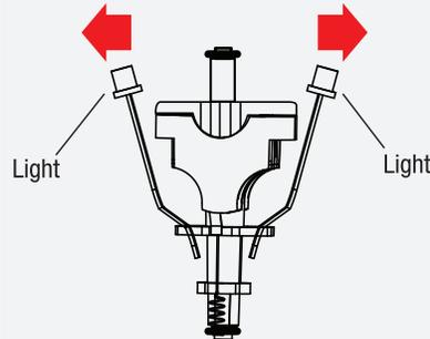
3. One at a time, carefully pull lights away from battery assembly.
