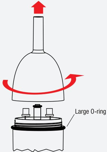
1. Unscrew top of float from bottom. Leave large sealing O-ring on threads in place.
