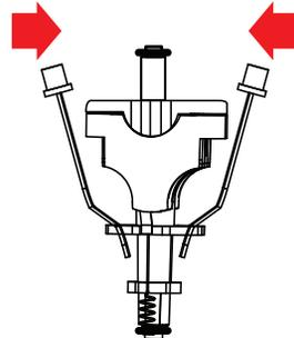
8. One at a time, carefully position lights back into cap.
